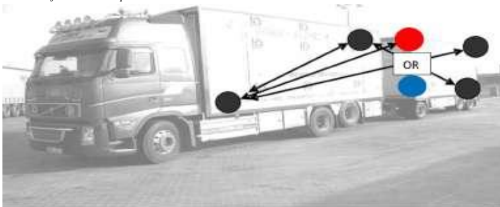
Position of the three temperature sensors in a multi-tier semitrailer
